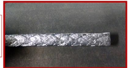
Once die formed, the Inconel® knit is no longer easily visible due to the carbon fiber strands pushing out the graphite up and over the Inconel®
